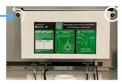
Lightbox is designed to tilt out - easy for fitting decals
