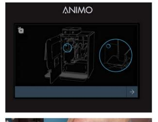
Close the machine, place an empty container below the outlet
