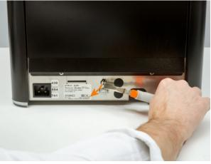
6 Locate the power pins remove the red and purple wire connectors
