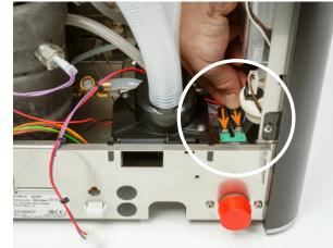
Guide the internal power cable to the opening in back cover and push through
