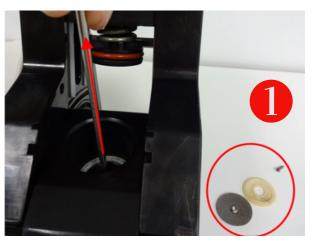
Use the brewer connecting screw to remove the lower piston from chamber
