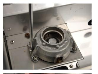
(10) Clean the rotating disc using a vacuum cleaner and the brush.
