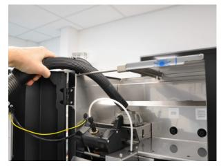
4 Loosen the screw on the top. Take away plastic outlet, sliding upper part away from grinder.
