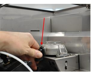
Fit bean hopper back into machine, fill with beans and open bottom slide.
