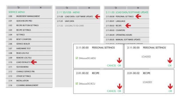
2 Remove the SD / USB from the slot.
