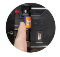
10 If you want to load the saved settings (recipes) in the machine, leave the SD / USB in place and follow the next Chapter: 3:Load Back Up Data.
