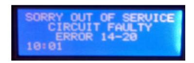
The error code 14 represents a circuit failure - Nothing more. The number after the hyphen represents the circuit with the issue/problem.
